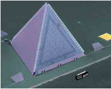
Figure 2: MEMS microphone is made by patterning plates in a plane and then folding them up by hand. The hinges on the edges are visible. Behind the open grill on the front is a membrane; it and the grill together form a capacitor. Sound moves the membrane relative to the grill and electronics (not shown) detect the changes in capacitance. (Courtesy of Flavio Pardo, Bell Labs, Lucent Technologies.)
