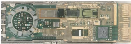
InP laser integrated on silicon photonic die
