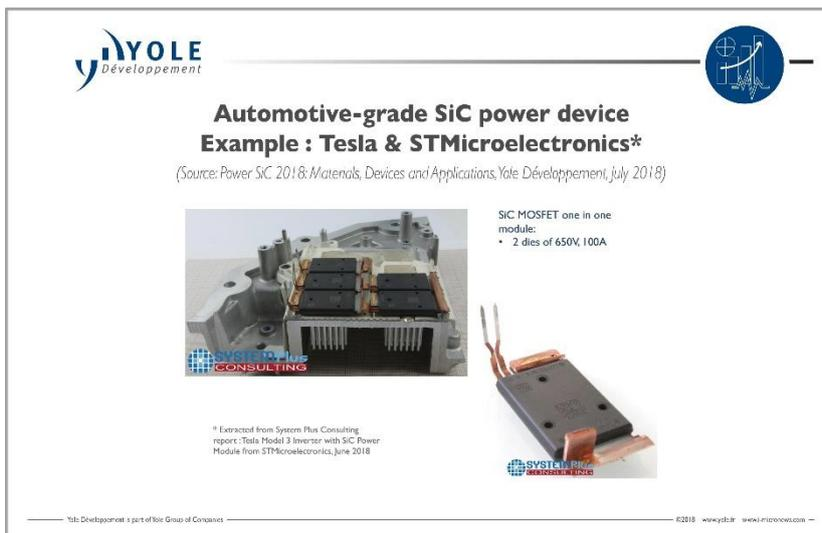
The recent SiC module developed by STMicroelectronics for Tesla and its Model 3 is a good example of this early adoption. The SiC-based inverter, analyzed by [System Plus Consulting](#), Yole's sister company is composed of 24 I-in-I power modules. Each module contains two SiC MOSFETs with an innovative die attach solution and connected directly on the
