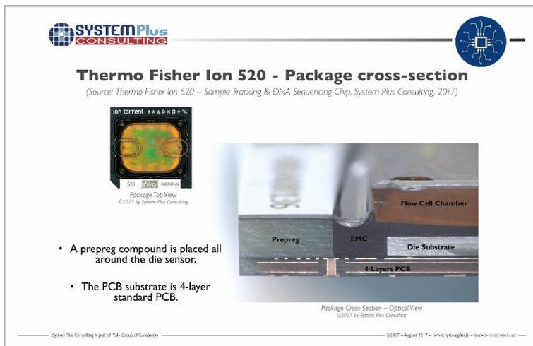
The innovative Ion 520 DNA sequencing chip uses this Ion Torrent technology. It includes a multiwell array, in which spherical particles that have DNA attached are trapped. The particles are sequentially flooded with solutions of nucleotides, which changes the charge in the wells when the introduced nucleotide is complementary to the leading unpaired nucleotide on the DNA strand. This results in pH change in
